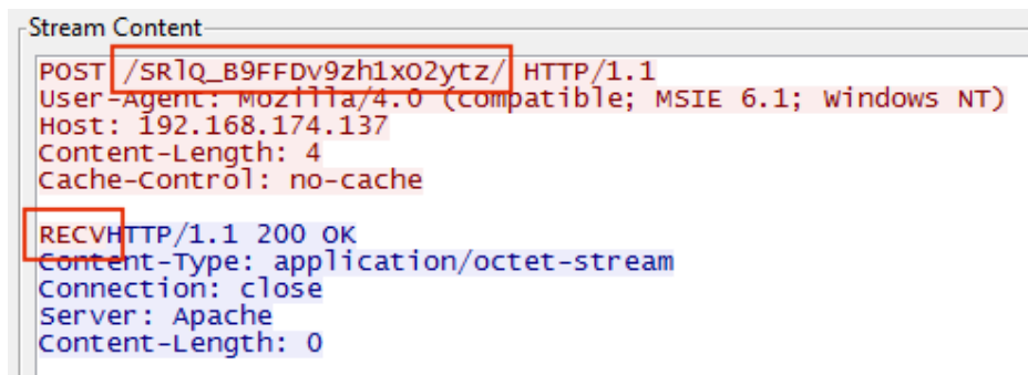
Figure 126: Packet details of meterpreter traffic
